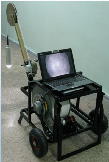
Unit with the automated cable winch
