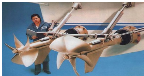
The boat movements : the semi-submerged screws of Arneson drive
