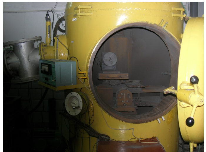
Unit for plasma spraying in the controlled environment
