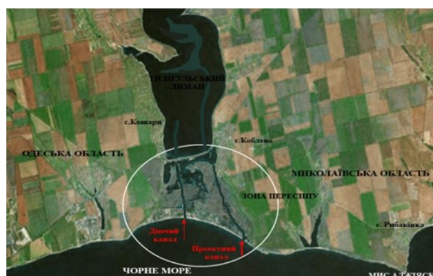
Placement of the existed and the projected channels on the filling of Tiligulskiy estuary
