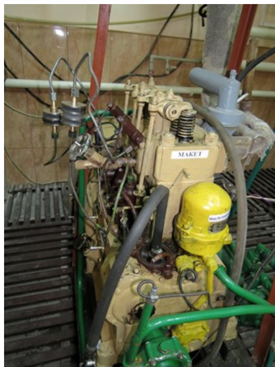
Picture 3 Stand for test of the magnetic actuators on the base of engine 2Ч10,5/13
