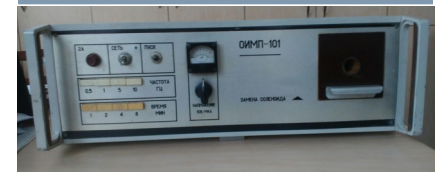
Picture 5 Unit for treatment of the fuel device pulse magnetic field OHMIT-101
