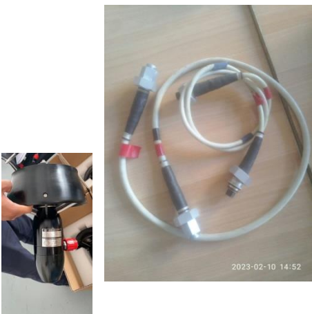
Underwater electric cables
